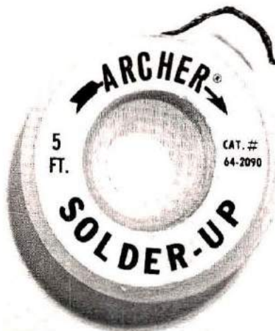
Solder-removing wicks are used in repairing PC boards or salvaging components. To use them, heat the soldered connection with an iron, and apply the tip of the metal wick. Solder is pulled up the wick, away from the component. After the tip has cooled, a section is cut off, exposing fresh wick ready for the next application (courtesy Radio Shack Corporation).
