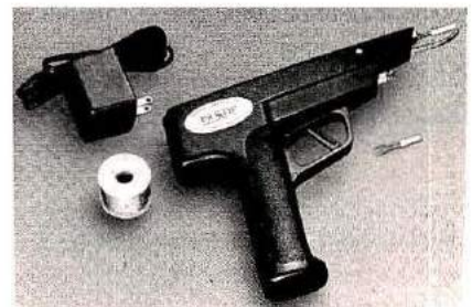
Cordless soldering guns, such as the Wahl unit shown here, can provide up to three times the "heat power" of regular cordless irons. This type of gun has a plug-in type of charger which can completely recharge a dead battery overnight. It also has a solder feed, and a choice of 16 different accessory tips (courtesy Wahl Clipper Corporation).
