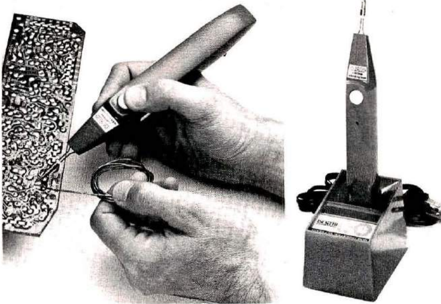
The new generation of cordless soldering irons provides great freedom from the ac cord that often hampered movement in delicate soldering operations. The very small tips available make the unit especially useful for densely packed construction projects (courtesy Wahl Clipper Corporation).
